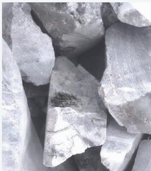
Figure 1 – Pakeagama Lake (PAK) Spodumene
