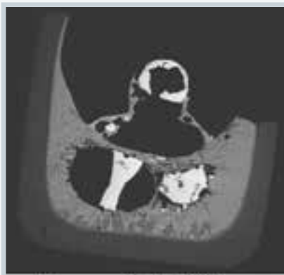
Figure 1 – Cross section of a 2g reduction melt producing metal and slag. Sample was drop-quenched from 1,550°C resulting in suspended metal phases.
