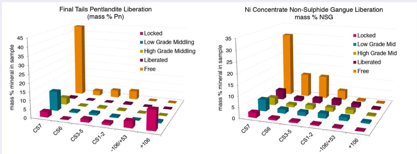
Liberation profile examples of free gangue slimes (CS7 or  $-3\mu\text{m}$ ) entrained to concentrate (left) and ultrafine (CS7 or  $-3\mu\text{m}$ ) free and liberated pentlandite losses to final tails
