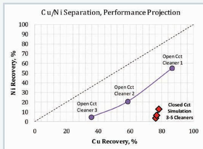
culated and compared to the closed circuit performance projections. Assessment of the liberation of the CuNi bulk concentrate allowed the construction of a theoretical grade/recovery relationship for CuNi separation, based upon perfect separation. At 76% copper recovery (based upon CuNi separation feed) the liberation data suggests that a Cu concentrate grade of approximately 32% Cu would be the maximum theoretically achievable.
