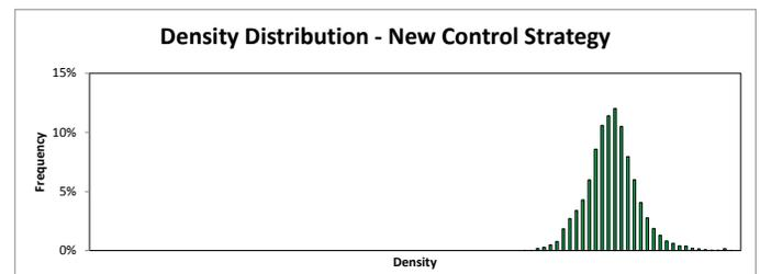
Distribution of density measurement comparing old and new control strategies; the standard deviation of density measurement is reduced with a process consistently operating at the higher end of the design limit.
