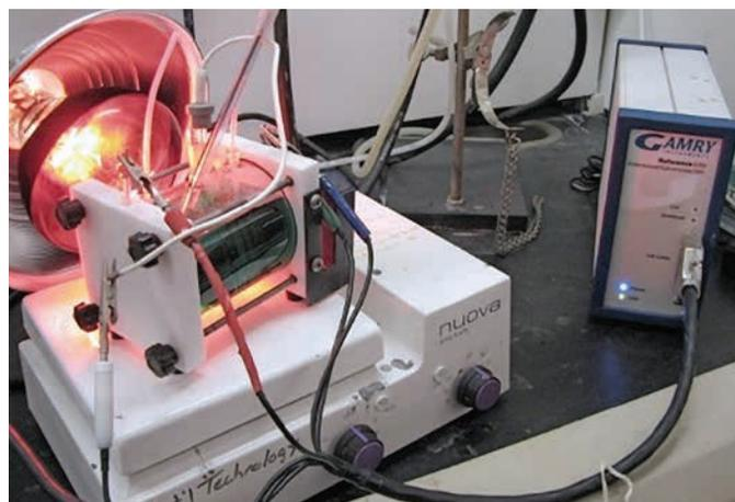
Figure 1 – Electrochemical setup used for corrosion testing
