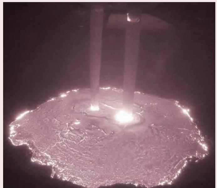
Still image captured inside a 1000°C furnace using a GoPro in a custom, air cooled enclosure.
