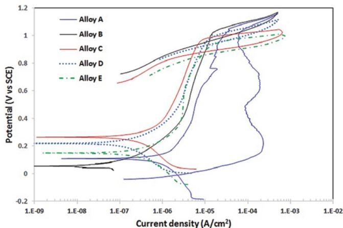
Figure 2 – Cyclic potentiodynamic voltammograms of the alloys at Condition 1
