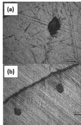
Figure 3 – Optical images of the pits formed on Alloy A (a) and Alloy B (b) after CPP tests at Condition 1
