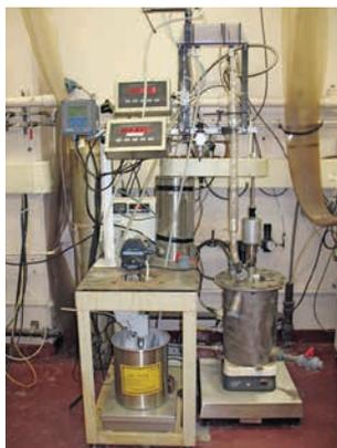
The Albion setup at XPS consists of an M4 IsaMill to efficiently produce the ultrafine ground ore or concentrate, followed by leaching in an agitated tank at atmospheric pressure. Fifteen kilograms of feed is required for determining the signature plot in the IsaMill, but a single Albion leach test can be carried out on as little as 1 kg of ground material. Typically, more
