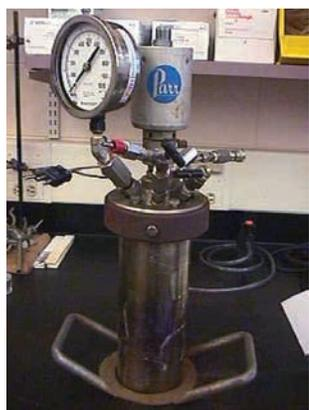
Pressure oxidation tests are carried out in a stirred 2L Parr bench-scale autoclave, which typically handles charges of approximately 1 kg. The autoclave is constructed of titanium and can be operated with an optional glass liner. It is fully automated to measure and control the temperature and pressure within the autoclave and the gas flow into the autoclave. The process
