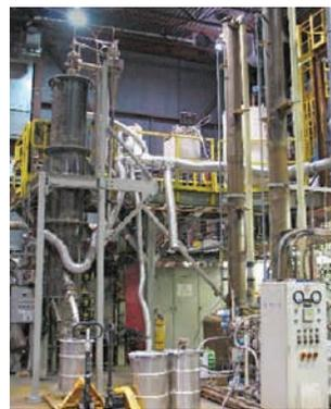
Comparative testing of all three options can be carried out at bench scale at XPS using the facilities and expertise on hand. Roasting can be completed in either 2”, 4” or 12” diameter continuous fluid bed roasters, each equipped with a cyclone, afterburner for combustion of arsenic and/or sulphur vapour, condenser, and
